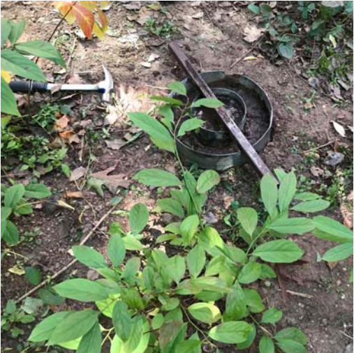
Testing infiltration rates among the Itea virginica. Courtesy of Rutgers MLA Program.
