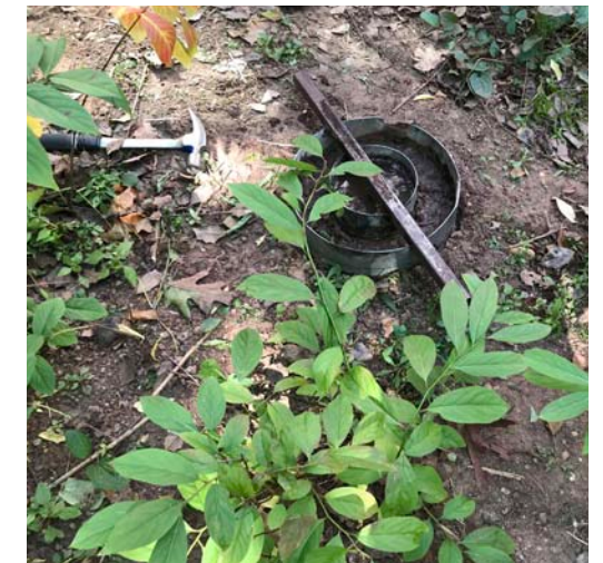
Testing infiltration rates among the Itea virginica . Courtesy of Rutgers MLA Program.
