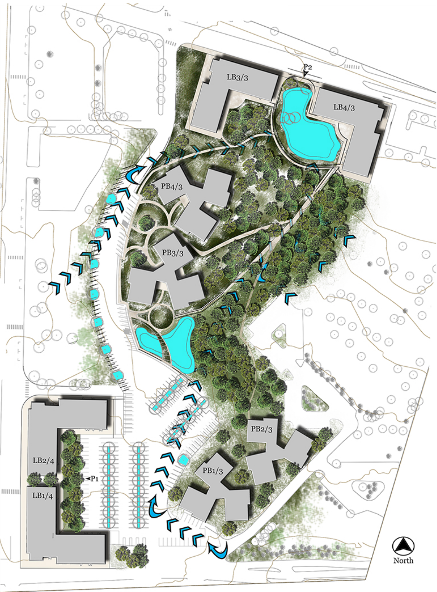
Post Development Plan - Sub areas denoted with blue catch stormwater run-off
