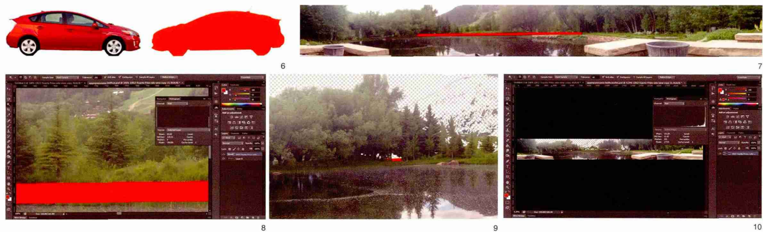
6 (a) 用于检验对临近道路视觉屏蔽效果的交通工具 (b) 使用颜色叠加后的图像 (a) Vehicle used to determine effectiveness of landscape buffer in blocking views of nearby road (b) the color overlay applied 7 汽车行驶轨迹图层位于全景照片图层之上 The line of travel swath layered atop the panoramic photograph 8 所选图层 (行驶轨迹) 的像素数 Pixel count for the selected layer (the traffic swath) 9 删去背景透露出行驶轨迹的可见部分 Removing the background revealed the visible parts of the traffic swath 10 直方图显示仍然可见的像素数量 Fig.10 The histogram reveals how many pixels are visible 11 使用 Kestrel 牌仪器收集国会谷住宅的气候数据 Using the Kestrel device to gather climatic data at the Capitol Valley residence 12 国会谷住宅的相对湿度、风速和温度数据在 ArcMap 中的内插值处理结果 Relative humidity, wind velocity, and temperature data interpolated in ArcMap for Capitol Valley residence 13 上午、中午和下午的人体舒适度图表 Human comfort chart in morning, afternoon, and evening
