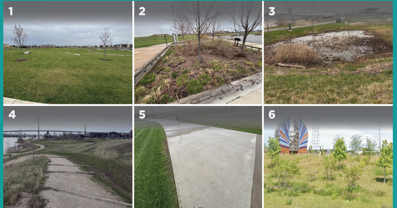
Figure 3.1: Different land cover types (in order: left to right, up to down): 1. Turf, 2. Garden Beds, 3. Stormwater Infrastructure (GSI), 4. Pervious Gravel Paths, 5. Impervious Concrete/Asphalt Paths, and 6. Dense Tree Plantings. Source: 1-5 taken on site April 10, 2026, Photo 6 Source: Google Earth
