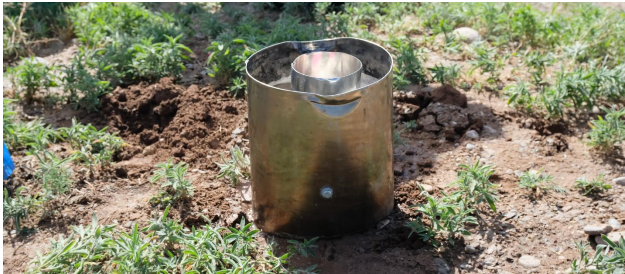
Figure 2.10 – The DIY double-ring infiltrometer showing signs of wear after repeated field use. This low-cost alternative was used to measure stormwater infiltration rates in both the garden and the adjacent untreated slope
