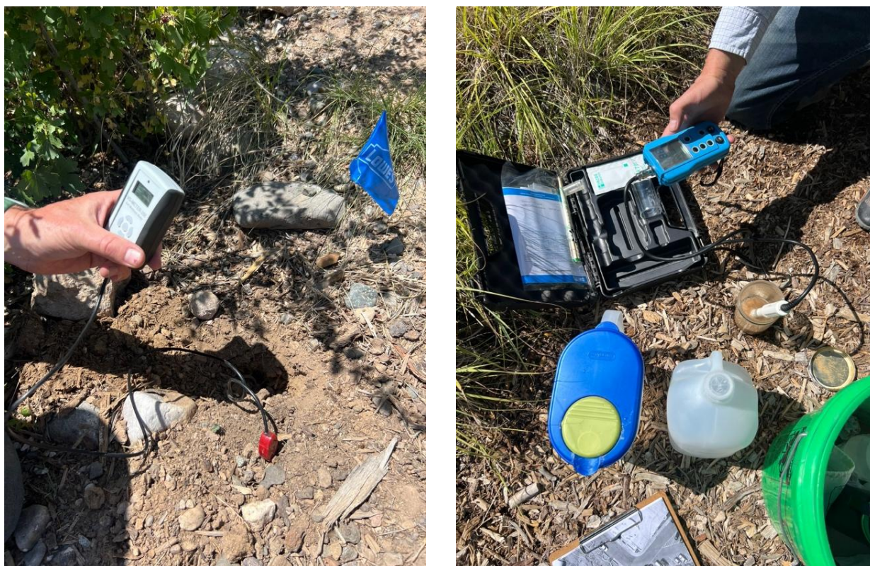
Figure 2.3 - Field testing on June 26 th . Left: Measuring soil moisture at ~4-inch depth using the Vegetronix VG-METER-200 sensor. Right: Preparing a 1:2 soil-to-distilled water slurry to test pH and electrical conductivity using the Hanna Instruments HI9811-51 meter.
