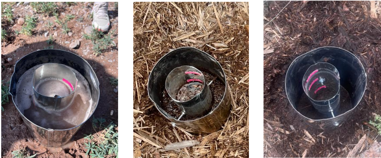
Figure 2.8 – (Left) Infiltration study test location map. (Middle) Test plot #2 in the upper contour swale of the EHFO. (Right) Test plot #3 in the lower orchard terrace of the EHFO.
