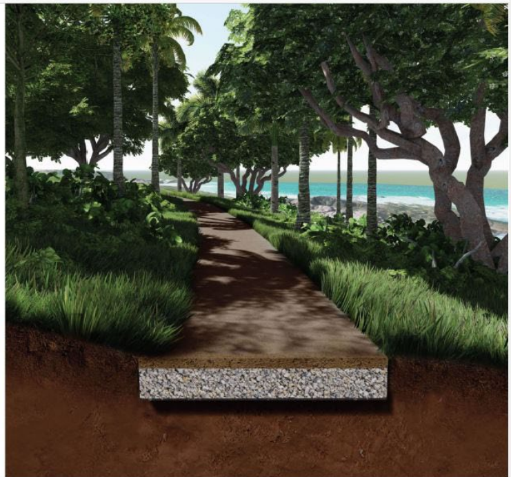
Figure 5. Design detail of permeable concrete. Source: EDSA
