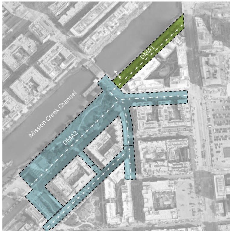
Figure 03: The area in green is Mission Creek Stormwater Park and is the current drainage area (DM 1). The blue area is the second drainage area (DM 2), stormwater from this area will be treated by the park once construction of the stormwater pump station is completed. Image Source: CMG
