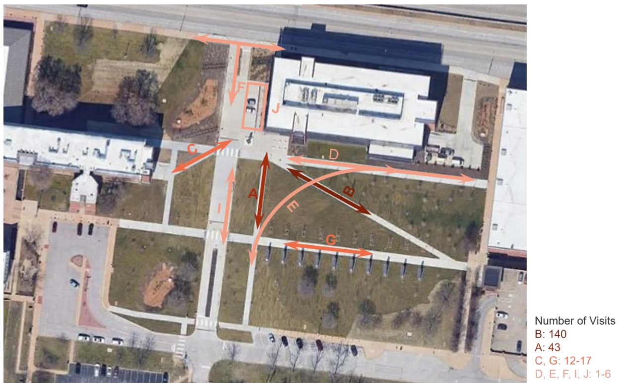
Figure 6. Routes of pedestrian movement by observation
