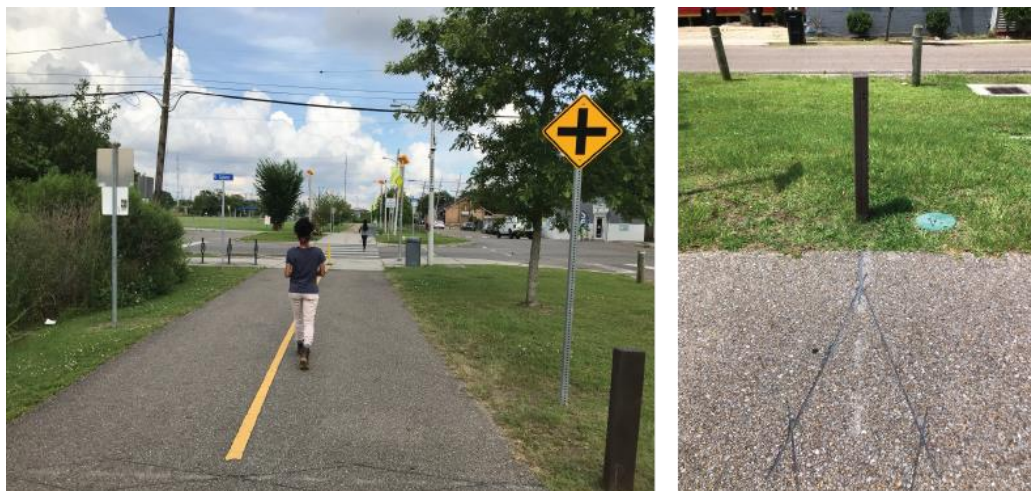
Figure 5a: Eco-Counter (brown post at the bottom right of the left photo) embedded in Lafitte Greenway trail at N. Galvez St. and St. Louis Ave. (Photo taken by the LSU CSI team.)
