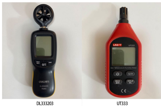
Figure 27 specifications and photos for the devices used for measurement of micrometeorological parameters
