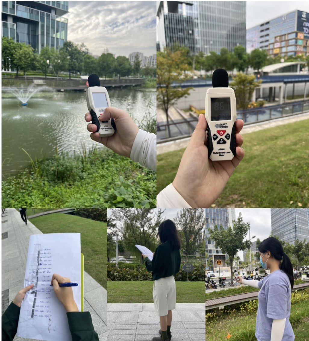
Figure 2.7: On-site photos during measuring the noise mitigation portion
