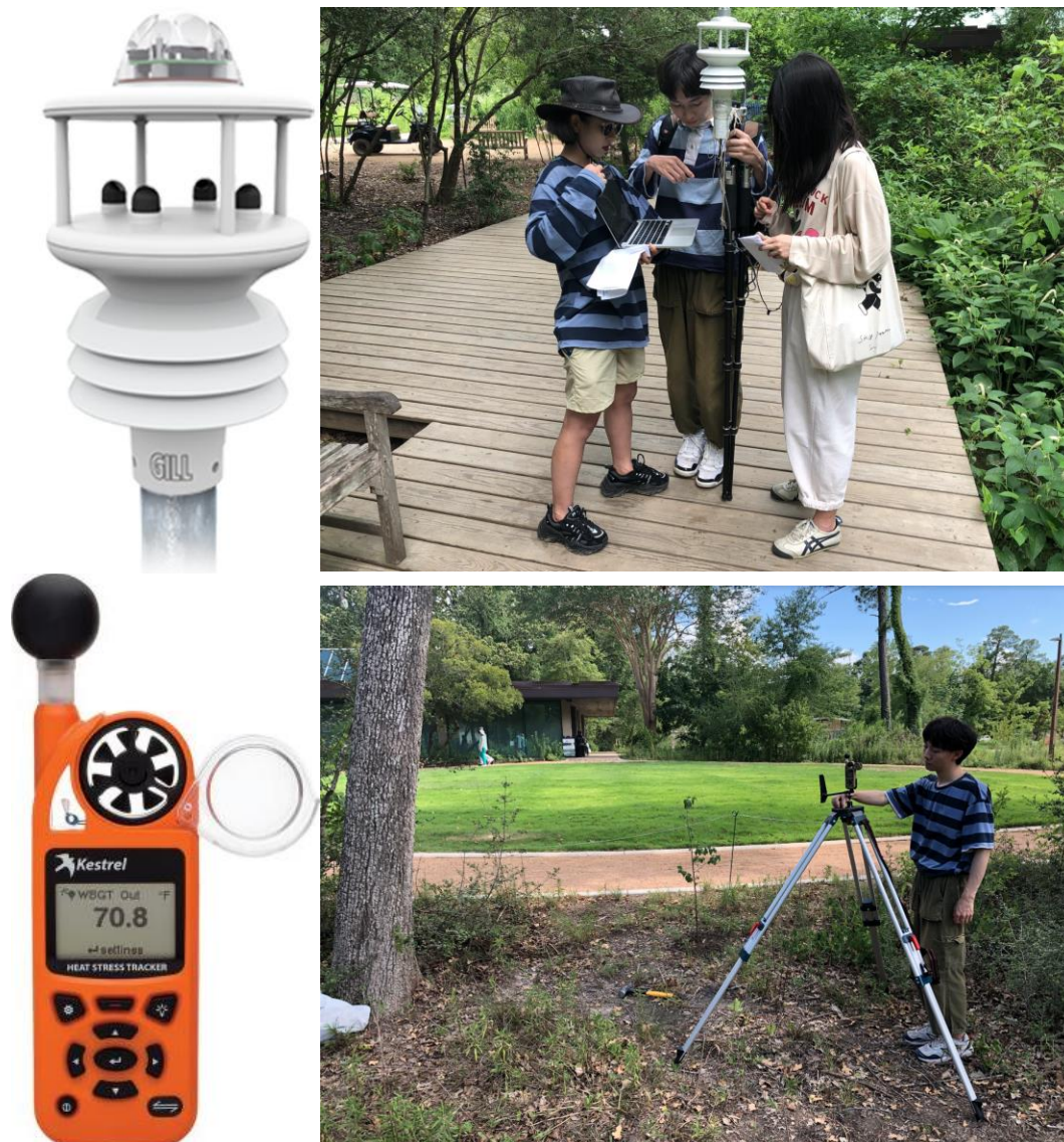
Figure 1. On-Site Microclimate measurements using MaxiMet GMX501
