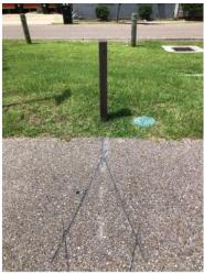
Figure 5a: Eco-Counter (brown post at the bottom right of the left photo) embedded in Lafitte Greenway trail at N. Galvez St. and St. Louis Ave. (Photo taken by the LSU CSI team.)
